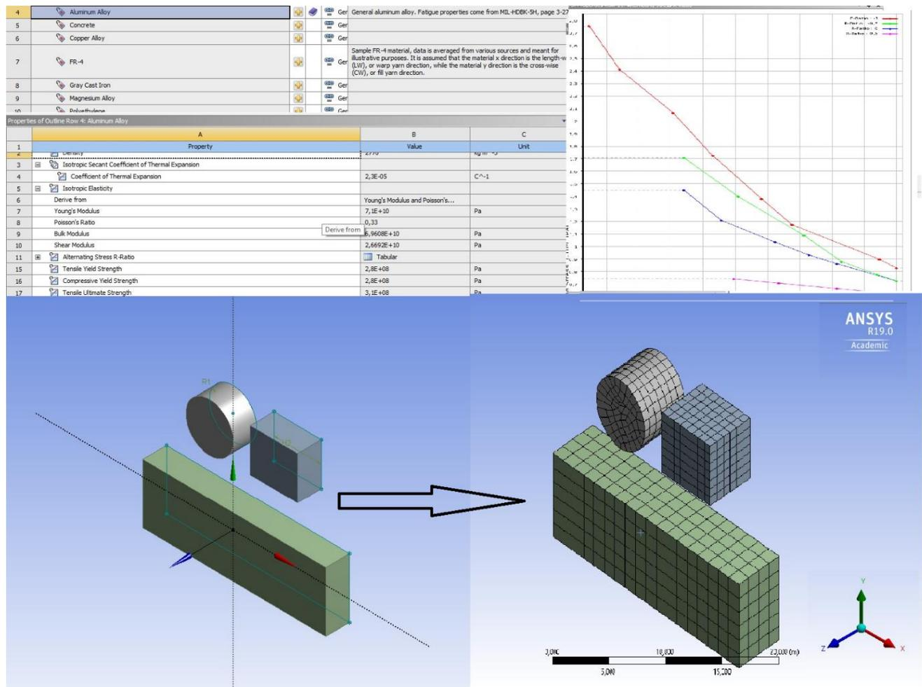
Figure 1 The mechanical properties of pure titanium, test samples, mesh test samples, and antagonist abrasive materials
