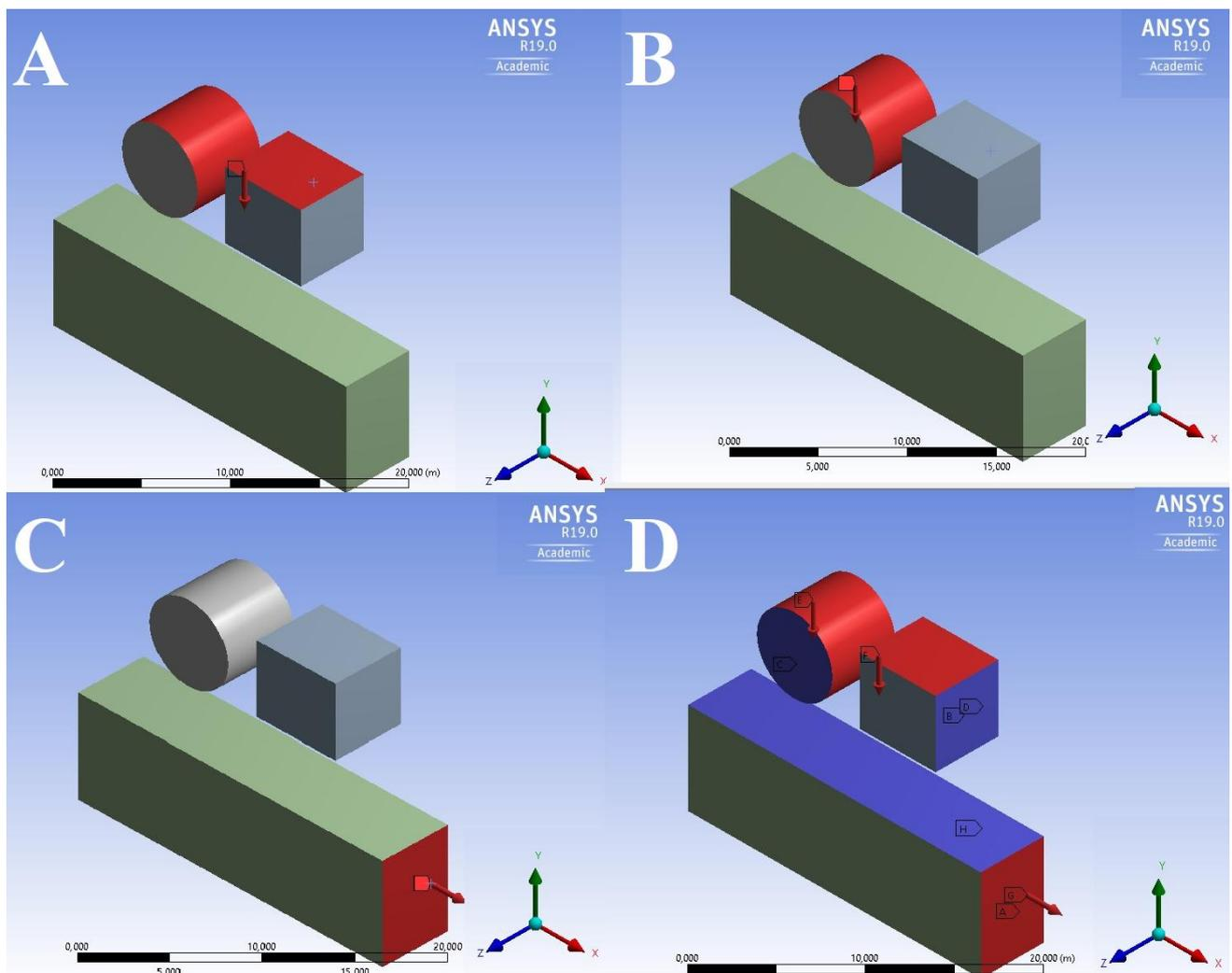
Figure 2 The process steps of chewing cycle test simulation movement. (A: Application of the bite force to the square counter material, B: Application of the bite force to the circular counter material, C: 0.7 mm lateral movement of the base test material at the moment of the bite force, and D: The effect of the test parameters on the materials at the moment of 1 cycle chewing movement
