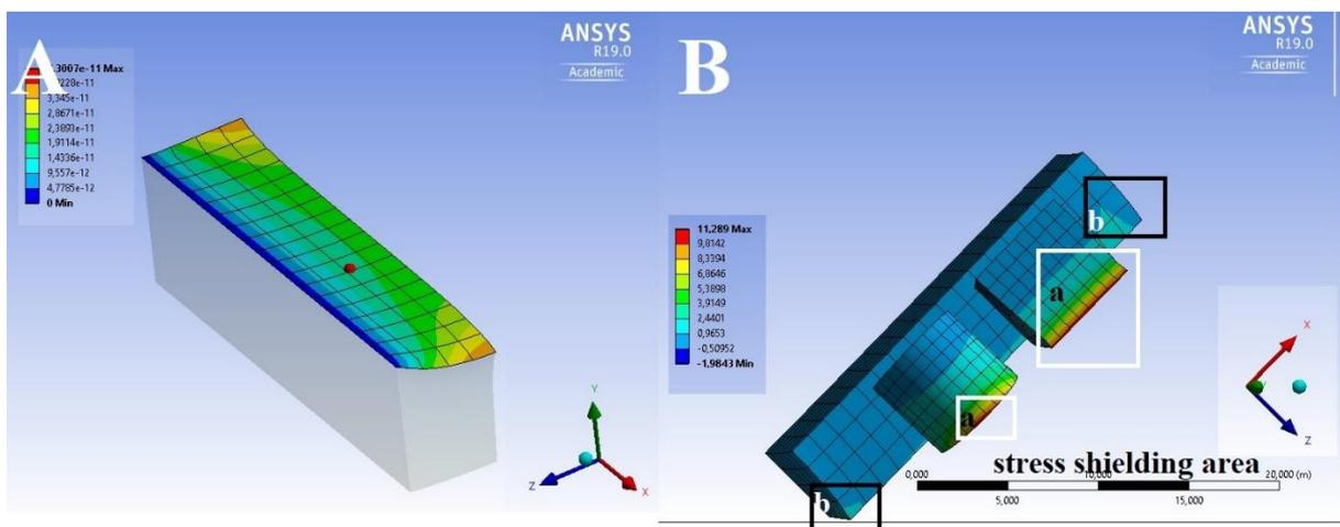
Figure 4 Two-body wear and stress shielding behaviors occurring on the test material and counter material during chewing (A: The two-body wear area on the test material that occurred during the chewing test simulation and B: The load distribution effect of the wear contact area on the antagonist abrasive material)
