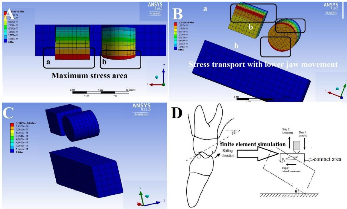
Figure 3 Chewing bite stress changes in the antagonist abrasive material during chewing movement (A: Maximum stress area both in antagonist material geometry, B: Stress transport with lower jaw movement, C: Chewing cycle is completed by separating the upper jaw from the lower jaw and D: The summary of the chewing simulation in the laboratory environment and on living tissue)
