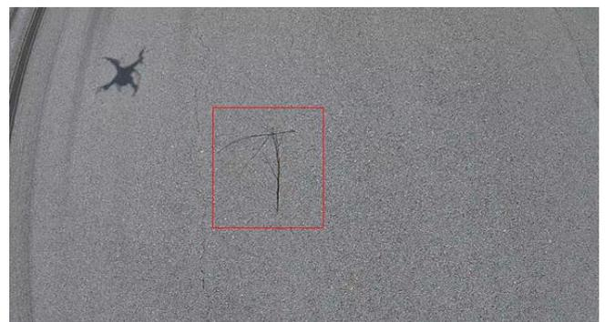
Figure 5 Foreign object (bush) detected on the runway
