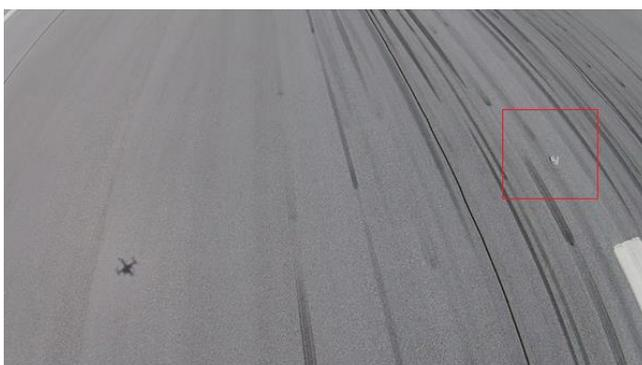
Figure 3 Foreign object (bag) detected on the runway
