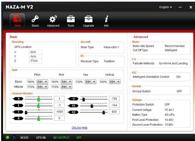
Figure 2 GPS position information input screen
