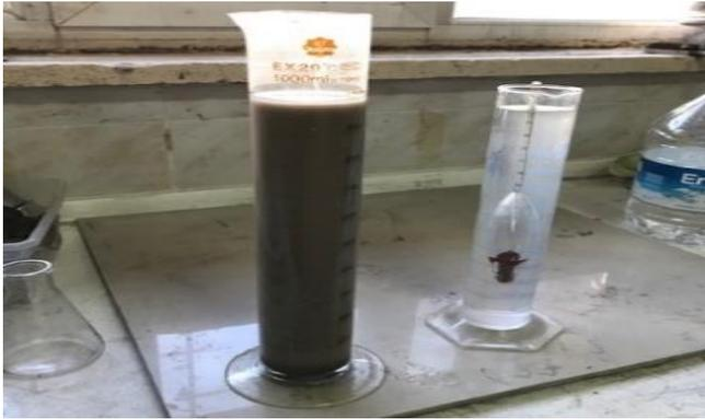
Figure 3 Hydrometer test setup.
