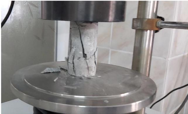
Figure 6 Fracture shape of cement and stone dust concrete in unconfined compressive strength test device
