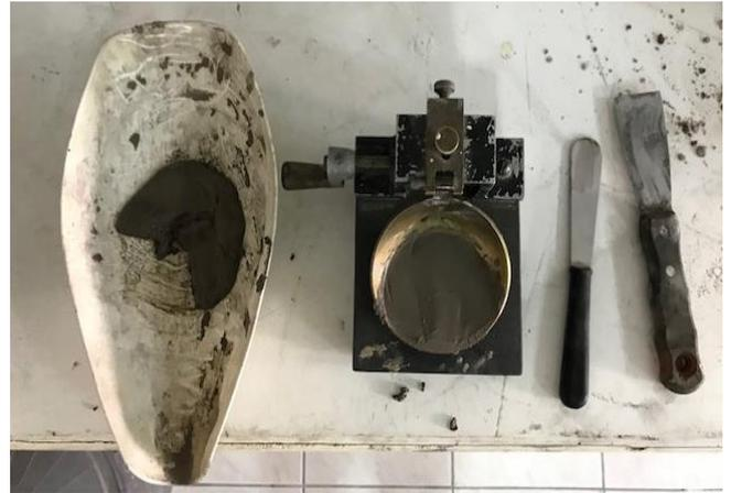
Figure 5 Liquid limit test (test setup in Casagrande)
