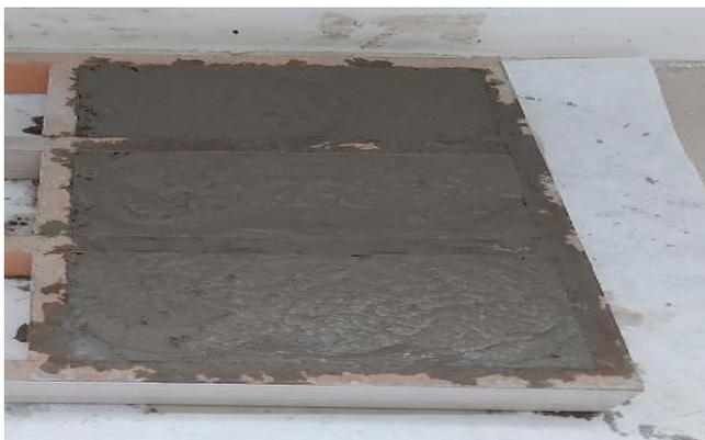
Figure 7 Cement + stone dust mortar prism samples
