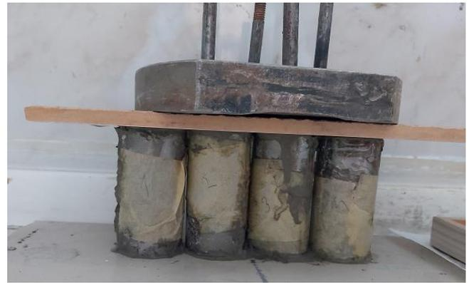
Figure 8 Cement + stone dust mortar cylinder samples and weights.
